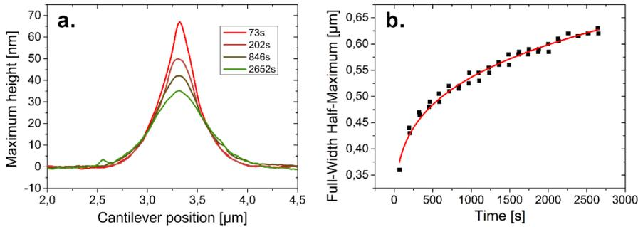
**Figure 4:** (a) Evolution over time of the bump profile generated on PPF<sub>10°C</sub>. (b) Data (dots) and fitting curve (line) of the evolution over time of the full-width half-maximum of the bump profile on PPF<sub>10°C</sub>
