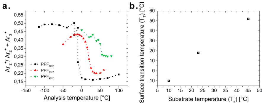
**Figure 5:** (a)  $Ar_2^+/(Ar_2^++Ar_3^+)$  ratio of backscattered ions collected during ToF-SIMS experiments versus the analysis temperature for PPF<sub>10°C</sub>, PPF<sub>23°C</sub> and PPF<sub>45°C</sub>. (b) Evolution of the  $T_T$  of PPF evaluated by ToF-SIMS as function of  $T_s$ .
