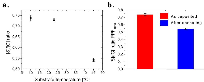
**Figure 6:** (a) Evolution of the S/C ratio as a function of  $T_s$ . (b) Evolution of the S/C ratio for the as-deposited PPF<sub>10°C</sub> and after annealing in air at 150°C during 1h.
