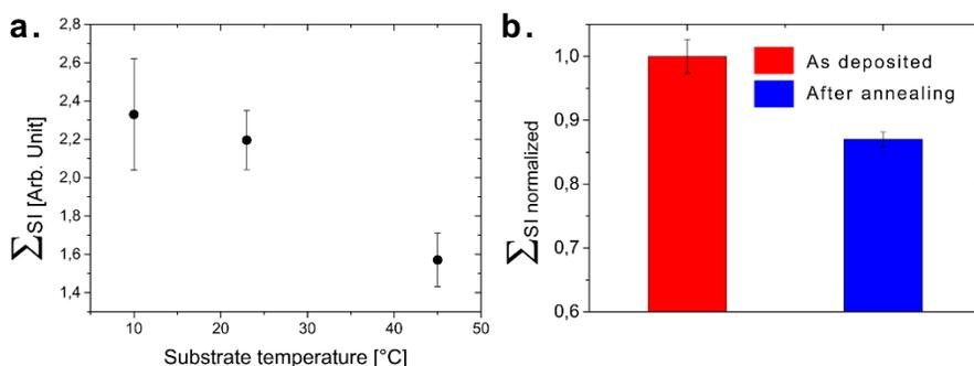
**Figure 7:** (a) Evolution of  $\sum_{SI}$  as a function of  $T_s$ . (b) Evolution of  $\sum_{SI}$  for the as-deposited PPF<sub>10°C</sub> and after annealing in air at 150°C during 1h.
