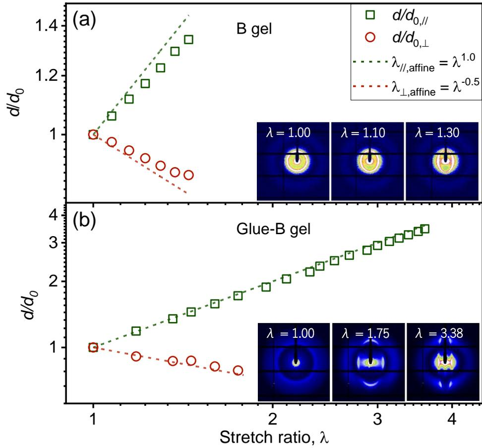
FIG. 2. Structure evolution of B and glue-B gels subjected to uniaxial tension as observed by *in-situ* SAXS measurement. The microscopic deformation ratio ( $d/d_0$ ) in the parallel ( $//$ ) and perpendicular ( $\perp$ ) directions of stretching versus  $\lambda$  for (a) B gel and (b) glue-B gel. The insets are the 2D SAXS patterns at representative  $\lambda$  for B and glue-B gels. Initial strain rate:  $0.01 \text{ s}^{-1}$ . Stretching direction is horizontal.
