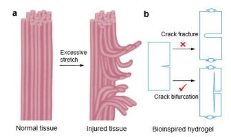
Figure 1. Biomimetic design of high-strength hydrogels. a, Simplified tearing model of fibrillar soft tissues 5-8 under excessive tension. b, Bioinspired design for crack-resistant hydrogels by deflecting the fracture along the stretching axis through crack bifurcation.
