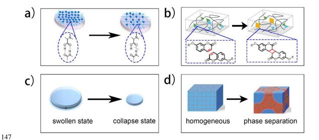
Figure 2. Mechanisms of hydrogels with responsive toughness. a) Noncovalent interactions. b) Formation or scission of covalent bonds. c) Volume change. d) Phase separation. Reproduced with permission.<sup>30</sup> Copyright 2020 Wiley-VCH Verlag GmbH & Co. KGaA.
