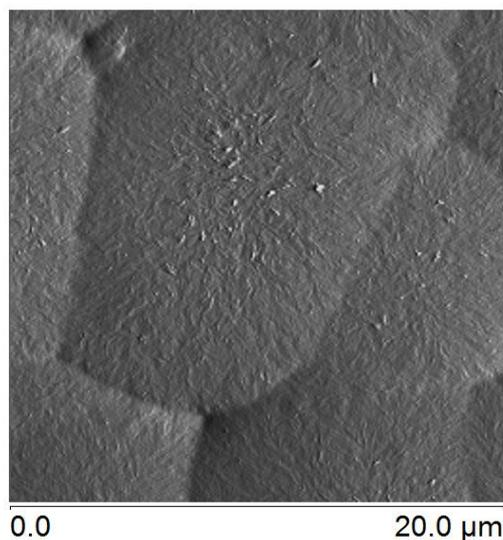
**Figure 11.** AFM amplitude error image of a blend with 60% PEKK and 40% PEI maximally crystallized at 250°C.
