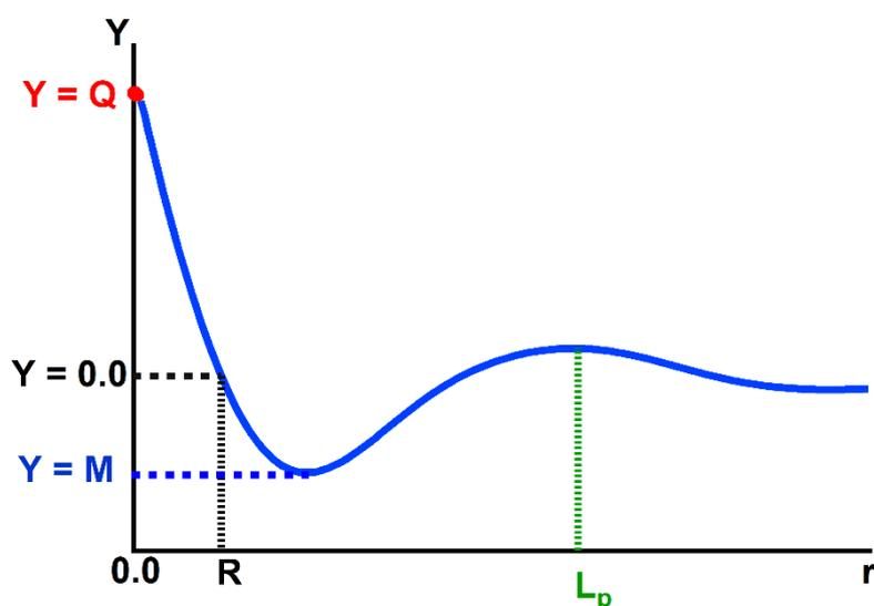
**Figure 2:** Example of the correlation function we obtained from SAXS measurements performed on our crystallized PEKK/PEI samples plotted as a function of the distance  $r$ . The characteristic points of the correlation function from which the lengths  $l_1$  and  $l_2$  involved in the lamellar stacks are determined are presented.
