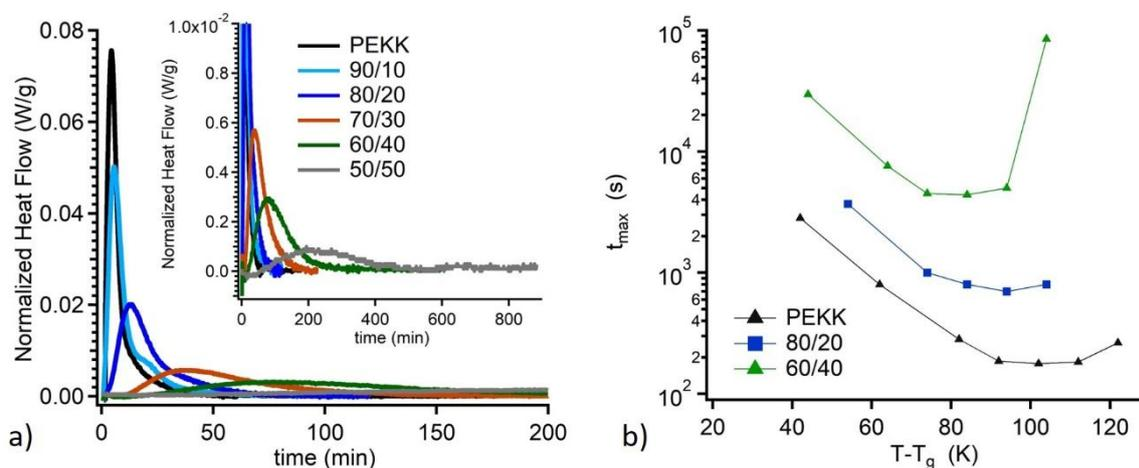
**Figure 8:** a) Time variation of the heat flow during the crystallisation isotherm at 250°C is plotted for various blend compositions (for the sake of clarity, an insert with a different time scale has been added). b) The time corresponding at the maximum of the heat flow variation during the isotherm is plotted as a function of the deviation of the isotherm temperature from the glass transition of the amorphous blend.
