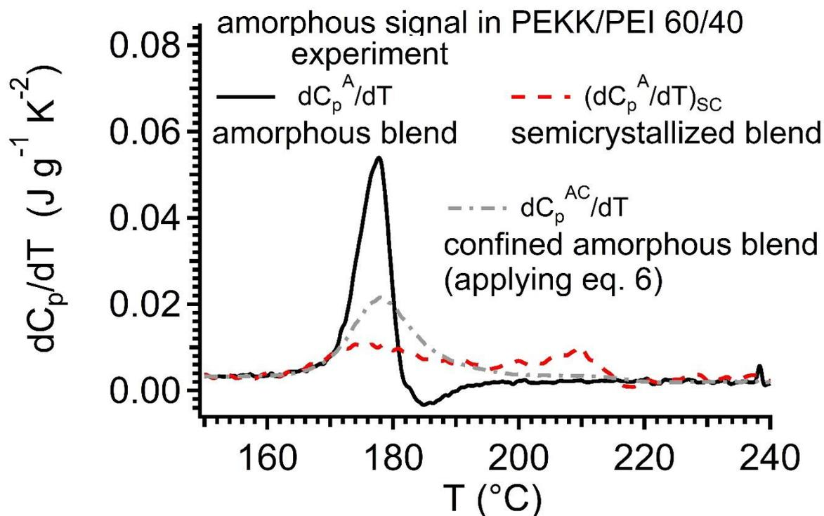
**Figure 16.** Heat capacity derivative  $\frac{dC_p}{dT}$  measured on 60/40 PEKK/PEI blends as a function of temperature. Data measured on amorphous and crystallized blends are compared. Signals for a confined homogeneous amorphous blend are deduced by applying equation 7 and assuming the  $T_g$  shift distribution that we determined for the amorphous phase in crystallized PEKK in Figure 15.
