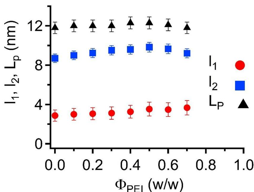
**Figure 10.** Variation in the characteristic lengths  $l_1$ ,  $l_2$  and  $L_p$  involved in the crystalline stacks of PEKK/PEI blends with the weight fraction of PEI,  $\Phi_{PEI}$ . The data result from SAXS measurements performed on blends maximally crystallized at 250°C.
