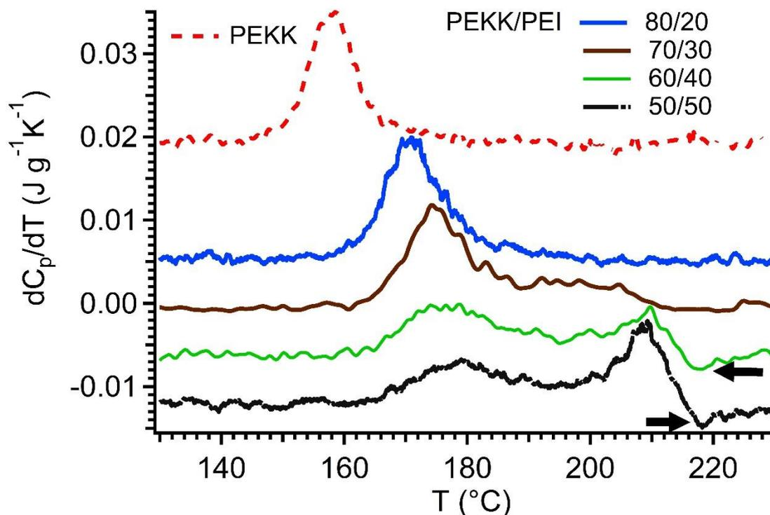
**Figure 13.** Temperature dependence of the derivative of the heat capacity with respect to temperature measured on PEKK/PEI blends maximally crystallized at 250°C for various PEKK/PEI blend compositions. Vertical shifts have been applied to the data for better visibility.
