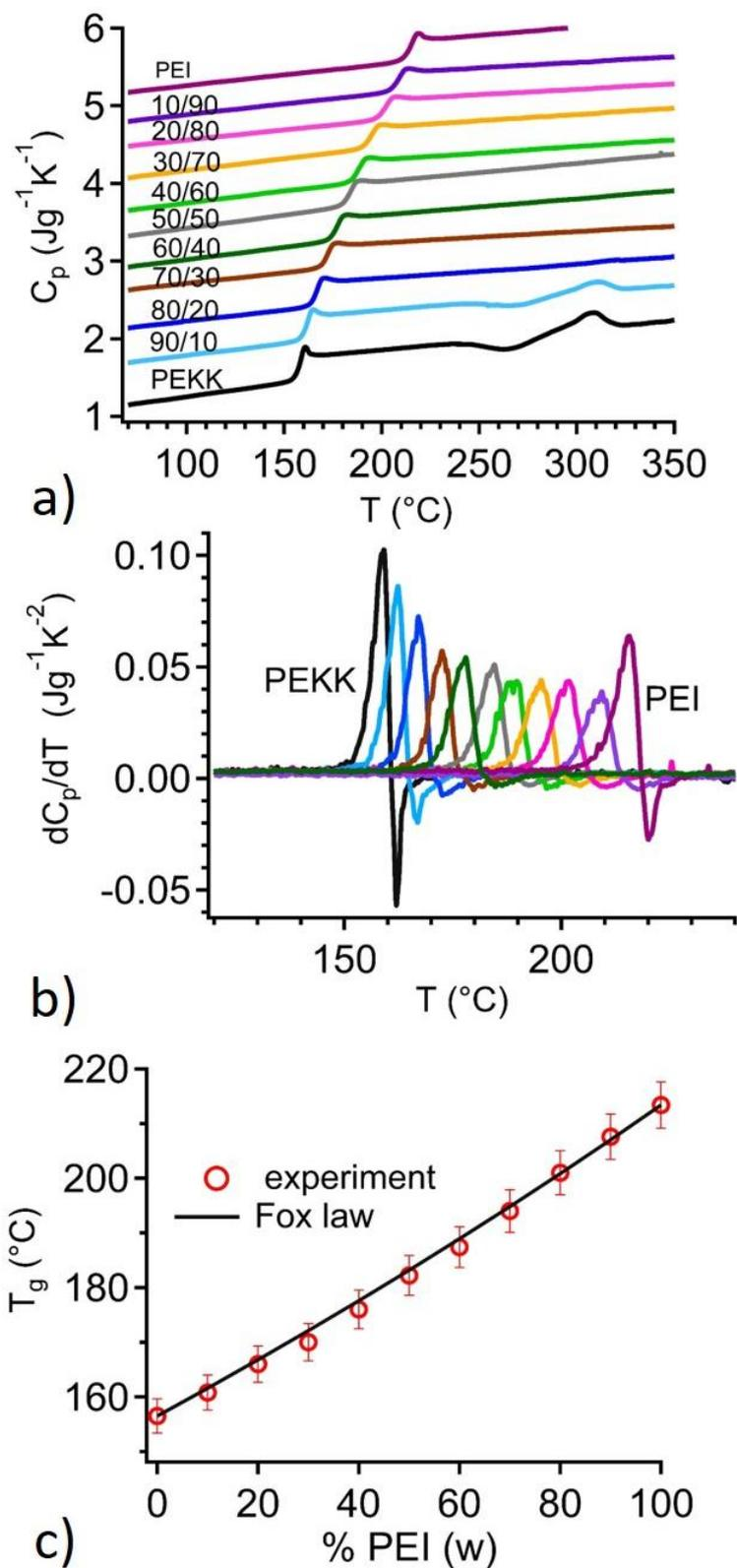
**Figure 4.** a) Variation in the heat capacity of PEKK/PEI amorphous blends  $C_p$  (in  $\text{J g}^{-1} \text{K}^{-1}$ ) with temperature of various compositions measured by applying a heating rate of  $10^{\circ}\text{C}/\text{min}$ . b) Corresponding derivatives  $dC_p/dT$  measured during the glass transition versus temperature for
