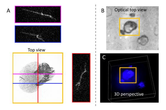
**Fig. S5.** (A) Confocal fluorescent microscopy of the biggest central cavity highlighted with a yellow square in (B) and (C), with corresponding cross-sectional images highlighting local crack bifurcation and tilt of cavity damage region. (B) & (C) are respectively the optical (in the maximum inflated state) and confocal (in the deflated state) view of overall Zone 2 identified in FIG 2.
