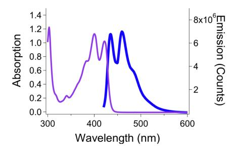
**Fig. S7.** Absorption and emission peak of  $\pi$ -extended anthracene moieties, data taken from [1]. Photoluminescence and excitation spectra were obtained from an Edinburgh Instrument spectrometer. The absorption spectrum was recorded between 320 nm and 450 nm for an emission at 460 nm. The emission spectrum was recorded between 420 nm and 600 nm, for an excitation at 405 nm. The reference molecule was diluted in ethyl-acetate at  $6\times10^{-5}$  mol.L<sup>-1</sup>.
