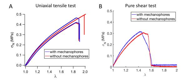
**Fig. S1.** Comparison of the mechanical properties of the ethyl-acrylate polymer network with or without mechanophores. No significant differences in elastic and fracture properties can be noticed both under (A) uniaxial tensile tests; and (B) pure shear tests.
