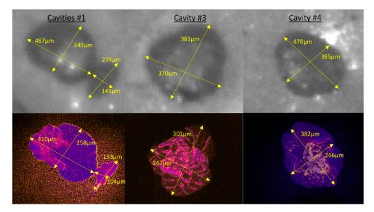
**Fig. S3.** Size comparison between maximum (inflated) cavity through optical visualization (top) and associated damage region, in the deflated state, visualized by fluorescent microscopy. The identified cavities correspond to the number-identification on FIG2A and are fortuitously well-aligned with the specimen xy-plane.
